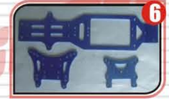
• Hardened aircraft grade T6 aluminum shock towers and upper deck
