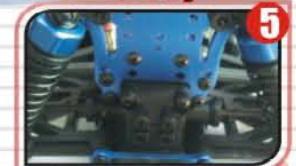
• Four wheel independent suspension, with oil filled shocks for better stability and handling
