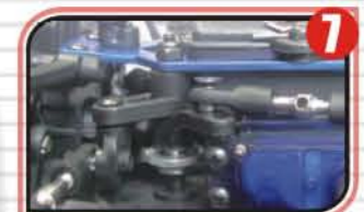
• Bellcrank steering with spring loaded servo saver
